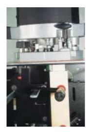
numerous tenon varieties (including useful twin tenons), square tenons may be routed by turning the templates around. Although, you will have to square the mortice ends with a chisel.
