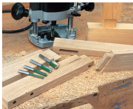
A selection of the joints that this jig can cut.
