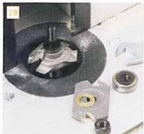
Use the scribed rail end as a guide to reassembling it all
