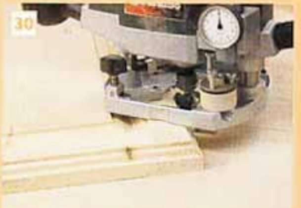
30 Run a suitable complementary mould round the outer edge to make it appear a little lighter
