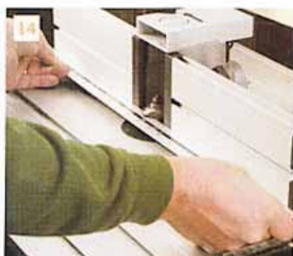
Make sure the fences of the table are in line with the bearing
