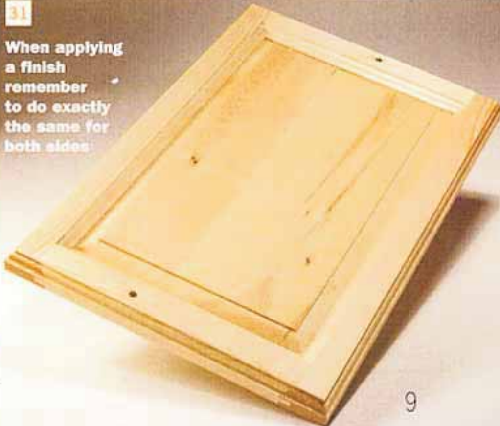
30 Run a suitable complementary mould round the outer edge to make it appear a little lighter
