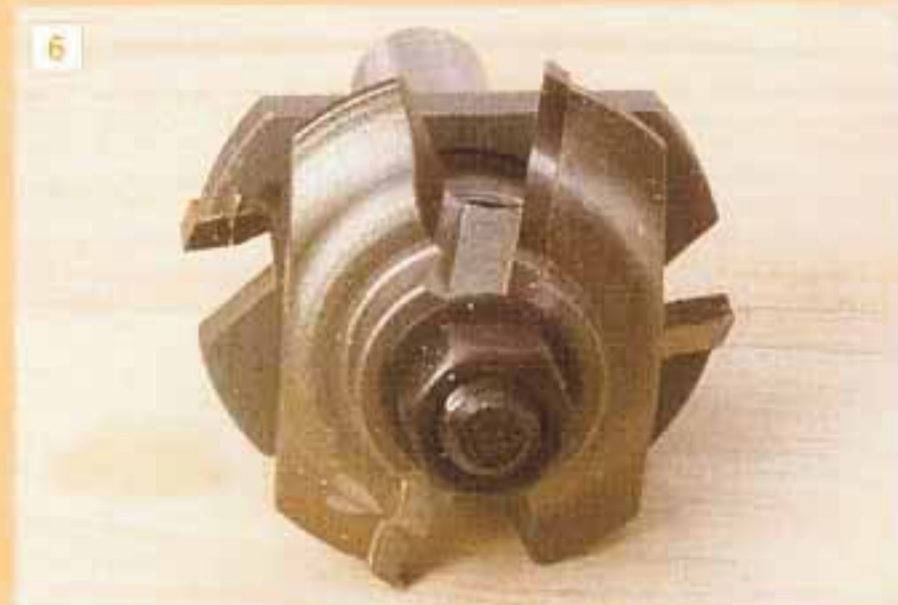
6 Make sure that each individual cutter is positioned at 90° to each other
