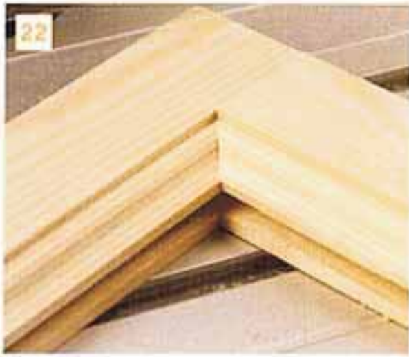
22 The rails and stiles should now fit together perfectly
