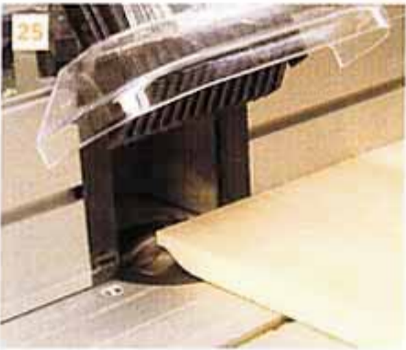
25 Make a shallow pass across the two ends of the panel
