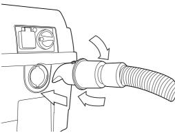
To remove bag undo the container hose deflector with hose bayonet cap by turning anti-clockwise and remove. Slide up collection bag. Close the bag by sliding the tab.
