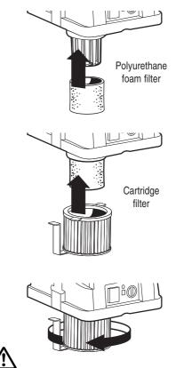
Before using the appliance always check that always check that all the filters provided are in the correct position.
