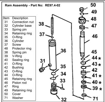
NOTE: Items marked with a "\*" are available as a Repair Kit - Part No RE97.4-RK, which contains items, 10, 11, 12, 13, 19, 23, 26, 39, 40, 41, 43, 44, 53, 57, 63, 65,
