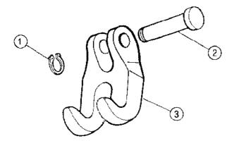
Item Part No. Description 184.C0010105 Circlip, D14 2 184.D5054700 Pin, D14x48x22 3 184.D2530500 Hook, Double
