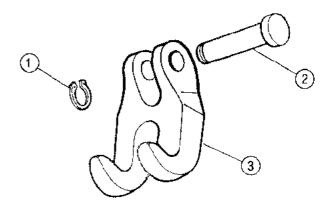
Item Part No. Description 184.C0010105 Circlip, D14 2 184.D5054700 Pin, D14x48x22 184.D2530500 Hook, Double
