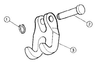
Item Part No. Description 184.C0010105 Circlip, D14 184.D5054700 Pin, D14x48x22 3 184.D2530500 Hook, Double
