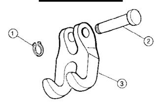
Item Part No. Description 184.C0010105 Circlip, D14 2 184.D5054700 Pin, D14x48x22 184.D2530500 Hook, Double
