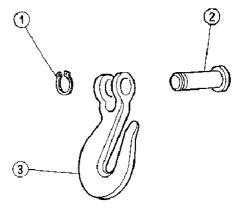
Item Part No. Description 184.C0010103 Circlip, D12 2 184.D5050100 Pin, D12x45x20 184.D2530100 Hook, Fork Ended
