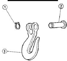
Part No. Item Description 184.C0010103 Circlip, D12 184.D5050100 Pin, D12x45x20 2 184.D2530100 Hook, Fork Ended
