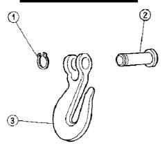
Item Part No. Description 184.C0010103 Circlip, D12 184.D5050100 Pin, D12x45x20 184.D2530100 Hook, Fork Ended
