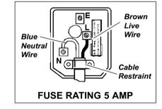
or replaced by a qualified electrician. When a BS 1363/A UK 3 pin plug is damaged, cut the cable just above the plug and **dispose of the plug safely**.
