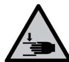
Warning crushing of hands
