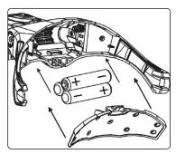
Open the battery cover and insert 3x AAA batteries (not supplied).
