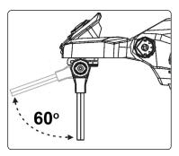
Adjust the angle of the lens.
