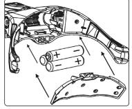
Open the battery cover and insert 3x AAA batteries (not supplied).
