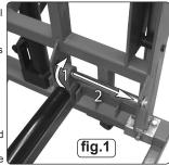
position, slide it along its hinge pin (fig.1.2) and lower it into the alternative locking positions.
