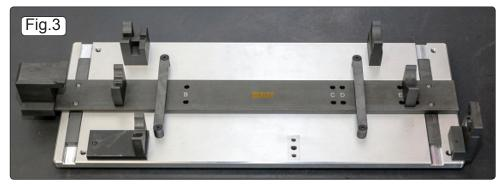
5.6.4. Place the inlet camshaft onto the VSE7171.04 and VSE7171.03 adaptors with the geared end facing the locking device (marked 13). Turn the inlet camshaft so the camshaft recess is facing outwards and slide the locking device (marked 13) into position, see figs.4 and 5.
