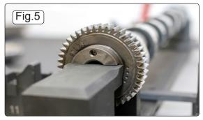
5.6.5. Place the exhaust camshaft onto the VSE7171.07 and VSE7171.15 adaptors ensuring the slot in the camshaft is facing upwards and the VSE7171.09 (marked 16) can be fitted and locks the camshaft into position, see fig.6.
