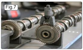
5.6.6. Using the VSE7171.06 Camshaft Locking Tool, (marked C2) ensure that the widest side of the tool is aligned with the widest side of the split drive gear. Tighten the VSE7171.06 until the teeth on the camshaft split drive gear are correctly aligned across the two halves, see fig.7.
