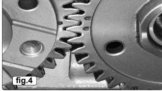
5.1.6. The timing marks on the camshaft gears must be aligned (fig.4).
