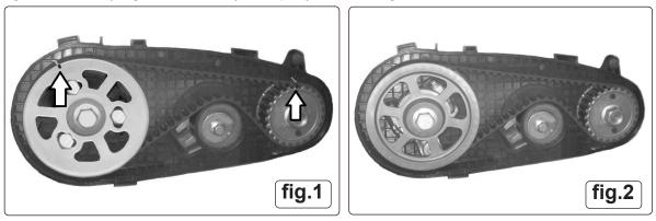
Fig.2 shows the later engine variant with fixed pulleys and no timing marks.
