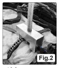
Fit the VSE4802-V2-01 link removal tool ensuring that the correct sized removal pin is used, fig.2.
