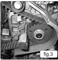
**NOTE:** It may not be possible to fit the VSE2092.06 Pump Locking Pin if the hub fork is slightly out of alignment; misalignment of 1-2mm at the pump hub is not detrimental to the engine's running and is considered acceptable.
