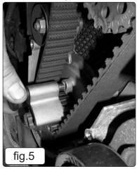
**NOTE:** Due to the gear design the locking tool has to be slid along the gear, and not placed over it. The lug of the Crankshaft Locking Tool must engage in the hole in the oil seal housing, ensure the timing marks are aligned. The timing marks on the two Crankshaft Locking Tools are not stamped in the same location.
