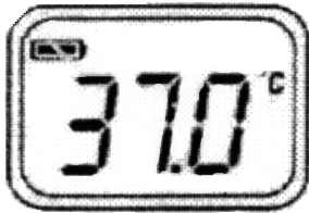
"Battery OK" - measurements are possible
