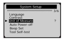
2) From **Unit of Measure** menu, use **UP/DOWN** scroll button to select the desired unit of measurement.
