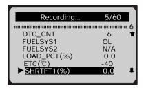
15) The scan tool keep recording PID data until user presses **ESC** button, the selected memory location is full, or it completes recording. A message prompting to playback data shows on the screen.
