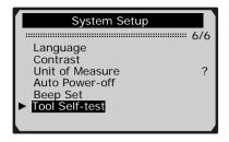
Select Display Test from Tool Self-test menu and press ENTER button.
