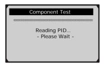
3) From **Component Test** menu, use **UP/DOWN** scroll button to select the test to be initiated.
