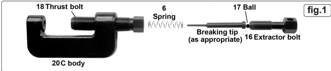
**NOTE:** If small 2.2 mm breaking tip is used you must also use the anvil (15) on end of thrust bolt (18) and anvil 2.2mm (12) at position Z on the C body (20) (see fig.2) to prevent breaking the tip.
