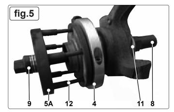
The force screw maximum torque is 150Nm. Exceeding this will shorten the life of the force screw. The force screw is considered to be a consumable item and is NOT covered under warranty.
