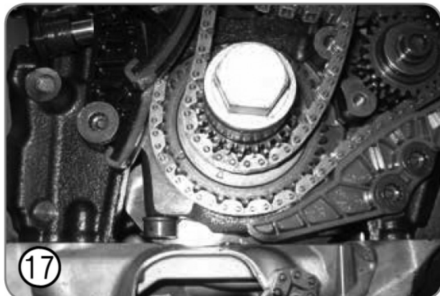
5.2.12. Remove the oil pump drive chain tensioner and detach the pump drive chain from the crankshaft sprocket.
