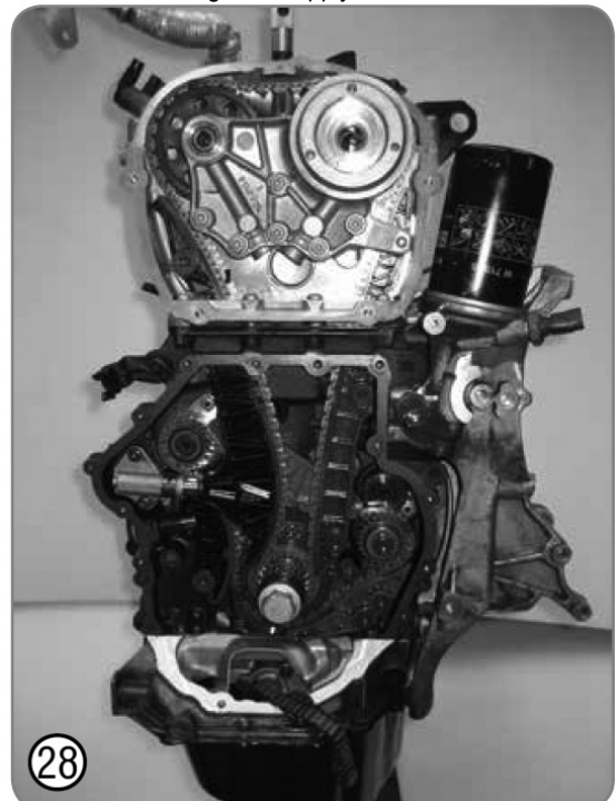
5.2.27. Ensure that the sealing surfaces of the cylinder block and the lower timing chain cover are clean and free from oil or used sealant.
