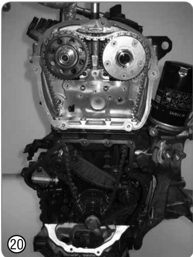
5.2.15. Remove the tensioner rail and guide rail for the timing chain. 5.2.16. Remove the timing chain.
