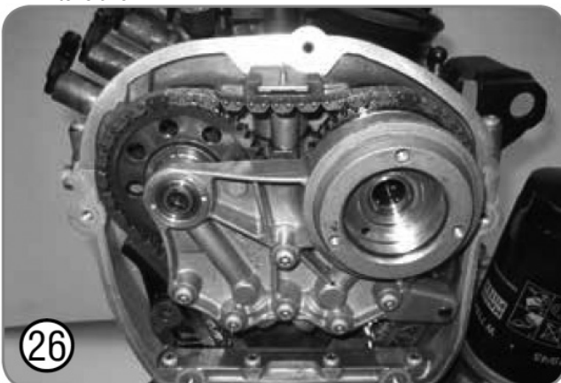
5.2.22. Remove VS5125-07 Chain Tensioner Locking Pin to apply tension to the chain. Ensure that the non-return block and retaining clip are fitted to the tensioner and operating correctly, it should not be possible to fully compress the tensioner.
