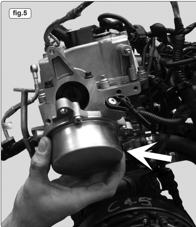
3.5. Remove the three retaining bolts from the vacuum pump, then remove the pump from the cylinder head.
