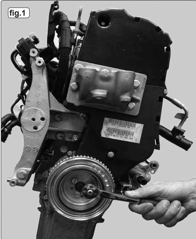
3.1. Remove the auxiliary drive belt and the crankshaft pulley.
