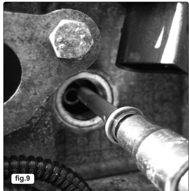
3.2.4. ALL Engines - Open sealing plugs and release the pins of the chain guide rails.
