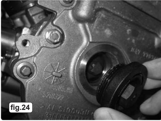
3.3.2. Remove the blanking plug from the engine (fig.24) to provide access to the pump sprocket centre bolt. **DO NOT** release the sprocket centre bolt at this stage.
