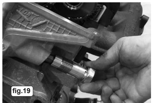
3.2.8. Remove the timing chain tensioner (fig.19).
