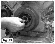
Fit the pulley on to the crankshaft and fit the split locking ring inside the bore of the pulley (fig. 13).
