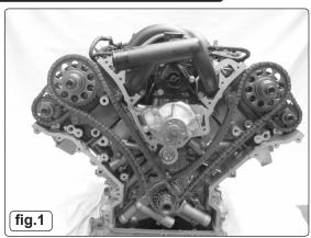
This V8 petrol engine was first introduced by Jaguar in 1997 and is still in use today. Land Rover also started to use the later versions of the engine in 2005. There have been many changes, both in engine capacity and components over the years, but most of the basic procedures for checking and adjusting engine timing, dis-mantling and assembly of the front-end gears, timing chain, camshafts etc., applies across the engine range.
