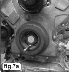
**IMPORTANT:** Insert the Thrust Plate into the centre hole of the pulley (fig.7).
