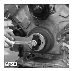
3.2.7 Prevent the crankshaft pulley from rotating by counter-holding with the VS4921 Tool. Screw in the Force Screw of the VS4922 Remover to extract the pulley off the crankshaft (fig.10).
