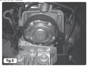
3.3 1.4 8v engine 350A1.000 with VVT (variable valve timing)
