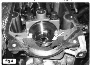
**NOTE:** The Setting Plate locates in to a "timing slot" in the rear of the camshaft (fig.4).
