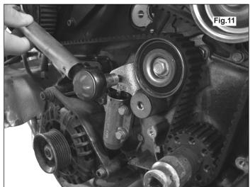
Fit torque wrench and 8mm hexagon socket bit to tensioner lever arm and apply 25Nm. torque in a clockwise direction. (Fig.11)
