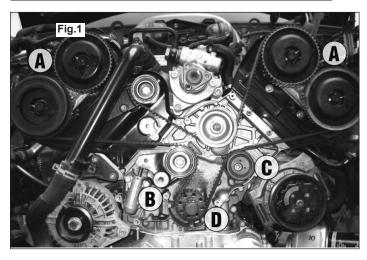
The VAG 3.0 V6 petrol engines are 'Quad Cam' engines with the timing belt directly driving all four camshafts from the crankshaft (Fig.1).
