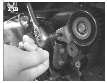
Apply pressure to the lever arm in an anti-clockwise direction until VS4593/1E Locking Pin can be removed. Remove the Pin to release the tensioner plunger. (Fig.10)
