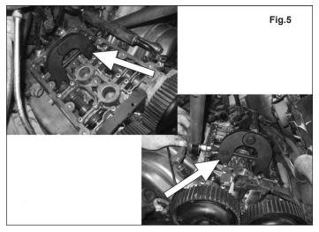
Fit one of the VS4941 Camshaft Setting Plates to the camshafts at **No. 3 cylinder** position on the left-hand bank (when looking from the camshaft sprockets), and the other Setting Plate onto the camshafts at **No. 4 cylinder** position, right-hand bank (when looking from the camshaft sprockets) (Fig.5).
