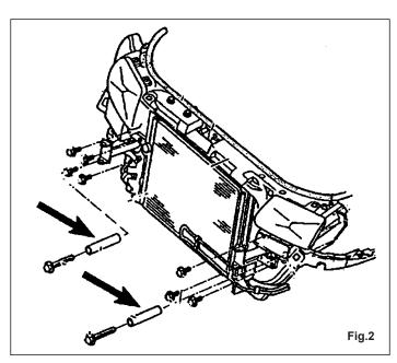
VS4741 Front Panel Support Guide Set Associated Tool – not included in VS4940 Kit
