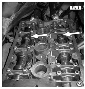
**4.1.2** Turn the crankshaft **clockwise**, using the centre bolt of the crankshaft, so that the lobes of the inlet and exhaust camshafts for No. 3 cylinder are **angled upwards**, (Left-hand bank, when looking from the camshaft sprockets). (Fig.3)
