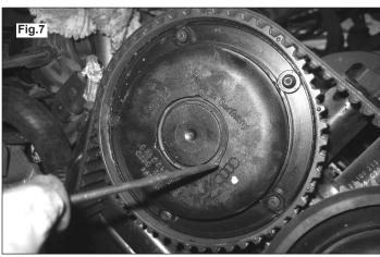
**4.2.2** Prise off the circlips and blanking plugs of all four camshaft sprockets, and slacken each camshaft sprocket bolt, leaving the bolt in place. (Fig.7).
