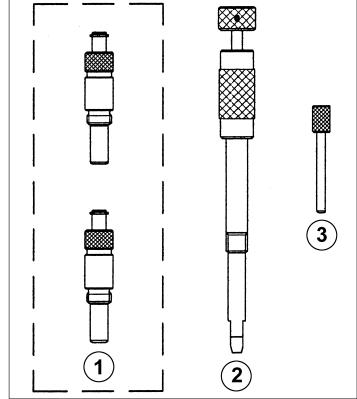
1 VS4926 Camshaft setting pins (pair)
