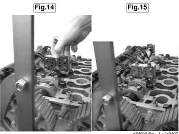
Using the Sprocket Holding Tool, make any final adjustment required to the camshaft position so the lobe aligns with the Setting Plates (Fig.16).
