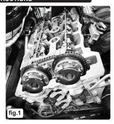
This range of 1.6 BMW 4 cylinder twin camshaft 16v. petrol engines have VANOS (VCT) units on inlet and exhaust camshafts but are not Valvetronic engines.
