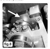
3.4.5 Place VS4868-1 Camshaft Setting Plate on to the rectangular section at the rear of the INLET camshaft, ensuring that the curved edge of the rectangular plate is uppermost. Align the camshaft so the Setting Plate rests fully on the surface of the cylinder head (Do not insert fixing bolt at this stage) (fig.8).
