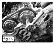
Slacken the bolts of the VANOS Units on the inlet and exhaust 371 camshafts (fig.16).
