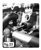
3.8.6 Attach a suitable torque wrench to the adjusting screw of VS4803 (fig.23) and turn to pre-load the tensioner rail to 0.6Nm.
