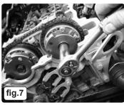
3.4.1 Slacken the bolts of the VANOS Units on the inlet and exhaust camshafts (fig.7).
