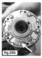
WARNING: It is important to note that the Inlet and exhaust VANOS Units are different. It is essential to keep the parts of Inlet Unit separate from the Exhaust Unit. Under no circumstances should the parts be mixed or parts from any other engine variant be used.
