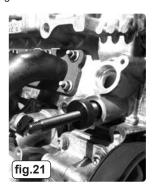
3.8.3 Insert VS4803 Tensioner Pre-Load Tool and screw in the adjusting screw by hand, until it makes contact with the tensioner rail (fig.21).
