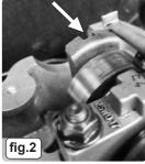
3.1.2 Check the timing positions of the camshafts – each camshaft has a rectangular section at the rear which has a curved edge on top and a straight edge on the bottom. With the engine in the correct TDC engine timing position, the curved edge of the rectangles, on both camshafts, will be uppermost (fig.2).
