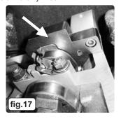
Place VS4868-1 Camshaft Setting Plate on to the rectangular section at the rear of the INLET camshaft, ensuring that the curved edge of the rectangular plate is uppermost. Align the camshaft so the Setting Plate rests fully on the surface of the cylinder head. (Do not insert fixing bolt) (fig.17).
