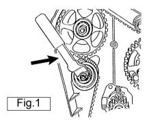
Fig.1 shows typical use of one of the specialised 'two pin' wrenches which locate in to two holes in the belt tensioner. Refer to the vehicle manufacturer's service instructions or a proprietary manual to establish the current procedure and data.
