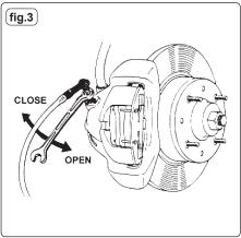
**NOTE:** Apply copper grease to the brake bleeding nipples before and after the brake bleeding procedure to reduce the possibility of seized or broken nipples when the brakes are next bled (fig.5).
