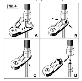
4.4 Clamp (Metal Fuel Pipe) - Use clamp to close off end of metal fuel pipe as indicated in fig.5.
