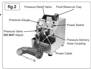
5.1.6. Remove the adapter from the open top of the unit reservoir and replace the filler cap. Further bleeding will not be required unless the bleed pipe is disconnected from the hose's quick fit coupling. The unit is now ready to use.
