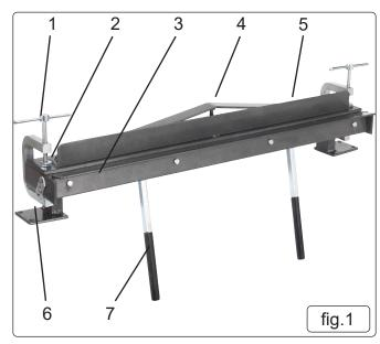
**4.10.** By rotating the end clamps through the vertical axis, longer lengths of metal sheet can be folded, i.e. fold a section, unclamp, move sheet, reclamp, fold second section etc.
