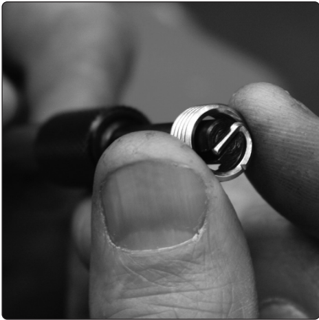
4.3 Load thread insert into installation tool.
