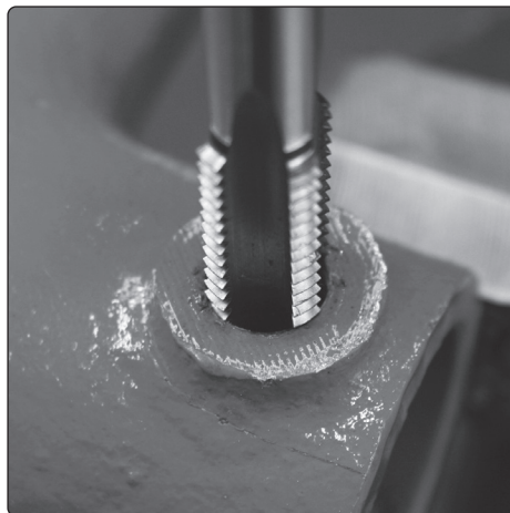
4.2 Tap drilled hole using screw tap provided.
