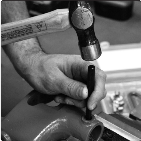
4.5 Remove the tag from the insert using the breaking pin tool.
