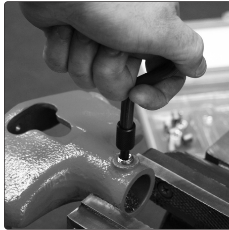
4.4 Screw insert into threaded hole.
