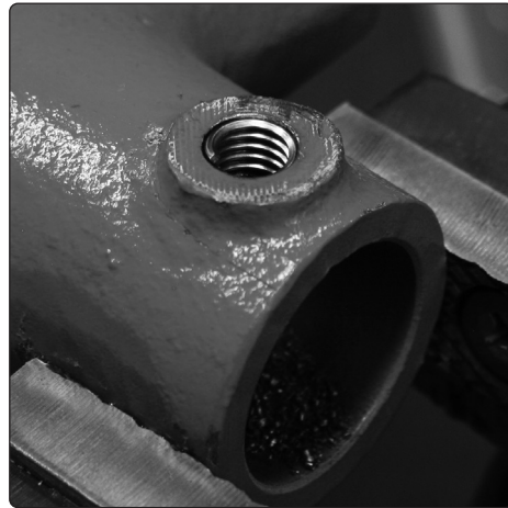
4.6 Thread is repaired and ready to use.
