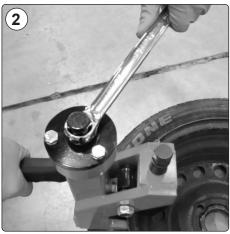
Turn the wedge foot drive bolt counterclockwise until it strips the tyre bead free of the rim
