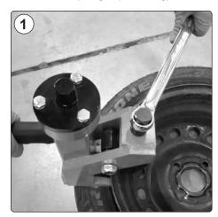
Turn the claw drive bolt counter-clockwise until the tool is in an upright position and the wedge is secured between the bead and rim. Use the handle to guide the tool.
