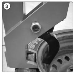
Retract the foot by turning the wedge foot drive bolt clockwise. Retract the claw by turning the claw drive bolt clockwise. Finally, remove the tool from the rim.
