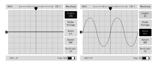
Figure 6 Waveform in GND couple status
