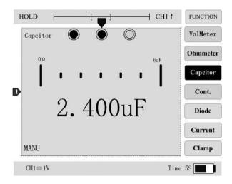
Figure 16 Capacitance Measurement Interface
