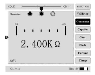
Figure 15 Resistance Measurement Interface
