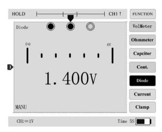
Figure 18 Diode Test Interface
