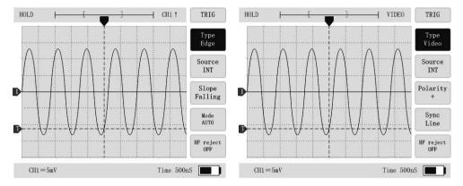
Figure 13 Trigger Interface
