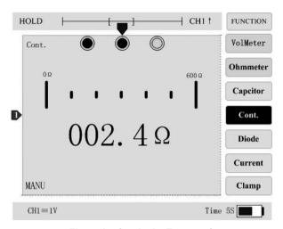
Figure 17 Continuity Test Interface
