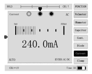
Figure 19 Current Measurement Interface
