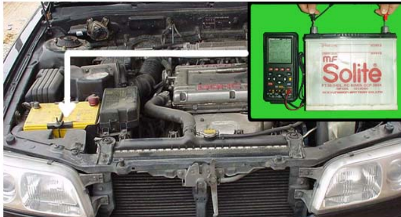
Battery location and test
