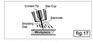
process is shielded from oxidising air contamination (fig.19). The shielding gas also assists heating of the weld. The torch is connected to the positive side of a DC rectifier, and negative clamp is attached to the workpiece.
