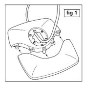
Your Tower Fan heater is supplied fully assembled with the exception of the base which comes in two halves. Please follow the assembly instructions carefully
