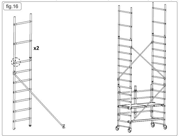
7.1.2. Install the boosters on the base of the scaffolding and assemble the lower diagonal attachments. Replace the 4 pins on the bottom of the booster so that they can be locked into the base.
