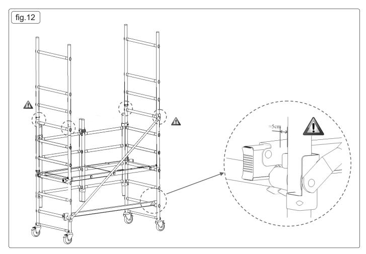
6.3. Assemble the 2 ladders on the base and attach the brace to the first rung (fig.12).
