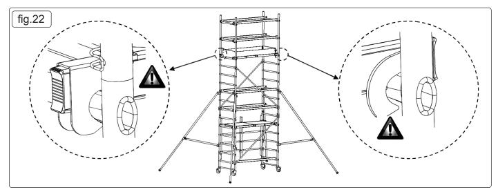
**9.3.** Start from the base assembled and attach the brace to the 1st rung. Prepare the '2 rung' and '7 rung' ladders removing the pins and stoppers from their bases.
