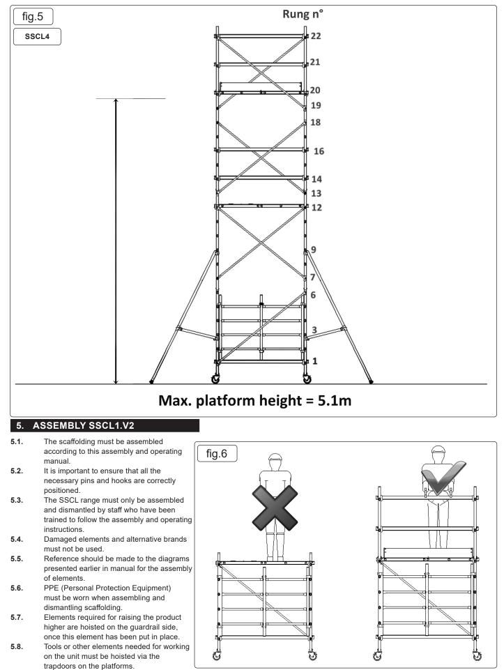
5.9. Never stand on a platform without protection (brace) when assembling high elements (fig.6).
