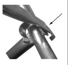
3. Rotate the fixing in the direction required for it to "clip" onto the standing support. This may require significant pressure which should be applied carefully and in a controlled manner to avoid potential injury to hands/fingers.
