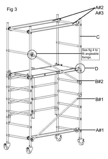
1. Place the fixing against the standing support. Ensure that fixing is perpendicular to the standing support. The rubber coated protrusion in the centre of the fixing, should be aligned with the appropriate tube in the standing support.
