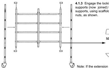
4.1.3 Engage the locking clip and affix the two side supports (now joined) to the two upright standing supports, using scaffold fixings and bolts M8 x 70 + 4x
