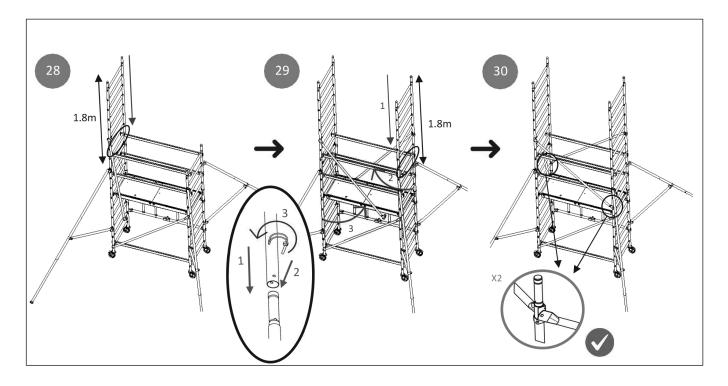
Fitting platform and rails Install the 2nd platform on the 13th rung refer steps 17 to 18, and place rails as shown in steps 20 to 23
