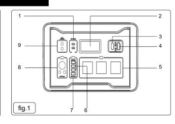
4.1. Charge the unit before first use. Connect the charge unit to a power source and insert the connector into either of the two 12v input sockets (fig 1, item 9). The LED will display current percentage charge stored and time required to charge to 100%.
