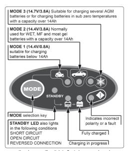
the charger will switch to float charge mode and will remain in this mode even if the user selects another mode. This protects the battery from being
