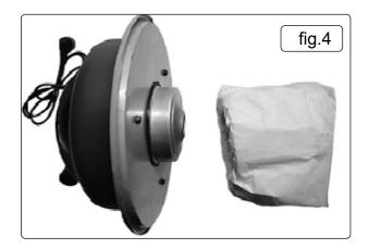
**5.1.3.** Plug assembled filter cartridge (9, 10) onto motor casing (1) (see fig.5).
