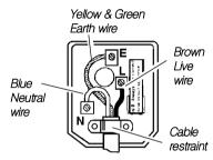
**FUSE RATING** THIS PRODUCT MUST BE FITTED WITH A
