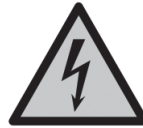
Electrical shock hazard
